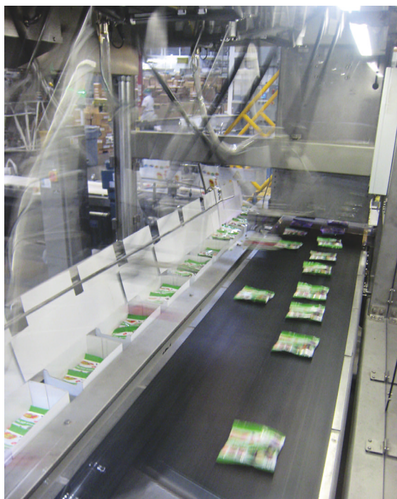
Three pick-and-place robots pick up bags of jelly beans from the incoming conveyor and place them into cartons. The system incorporates a vision system that locates the bags and directs the robots.
