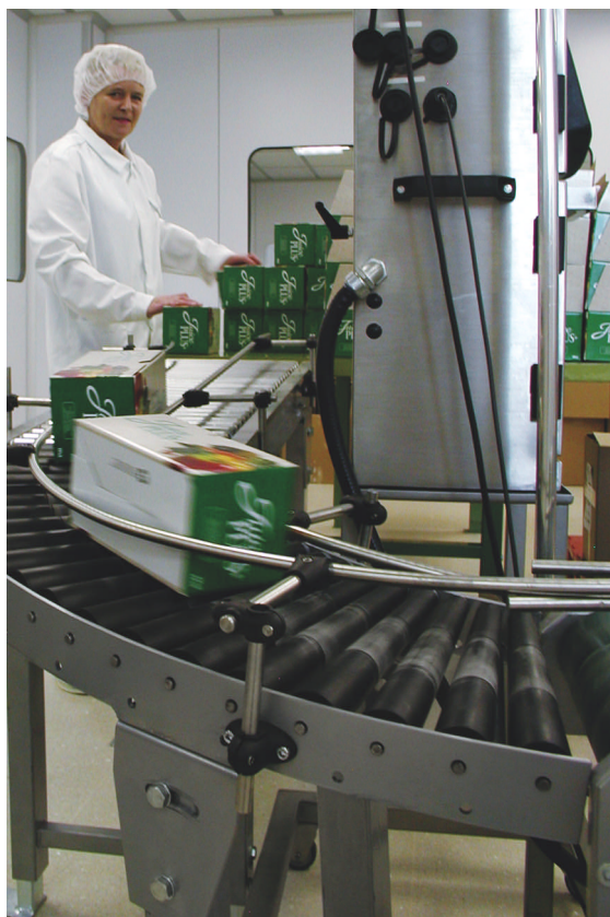
A line sends filled corrugate boxes down a conveyor. The boxes' auto-bottom design (seen against the conveyor track) enable quick and easy pack outs.
