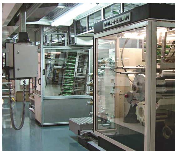
The bottles are printed by Exal, using a clear basecoat followed by eight colors and a glossy overfinish.
